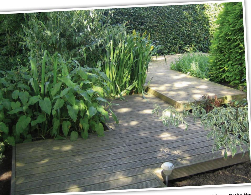
Elevated boardwalks preserve underlying existing vegetation & drainage conditions. Paths that are not high off the ground may not preserve underlying vegetation, but leave soils undisturbed and better able to soak up rain water.
